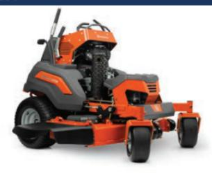
The balance of power and compact size make the V554 a serious contender in the commercial stand-on market. A robust frame, 7 gallon capacity and commercial 7 gauge cutting deck maximize durability and productivity.
